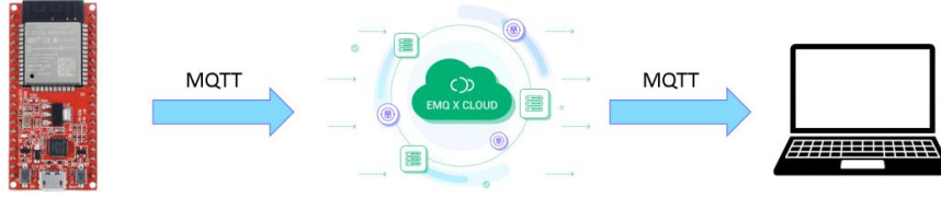
Figure 9: Data transmission pipeline. The above diagram shows the communication between the ESP32 MCU, EMQ X MQTT broker, and the computer. Sensor data are published to the EMQ X server and subscribed by the computer for real-time processing and analysis.
